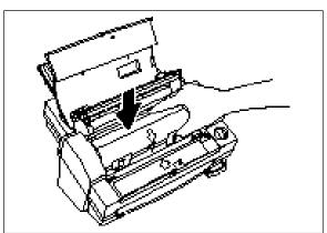
(7) Set the film cartridge into the machine.
